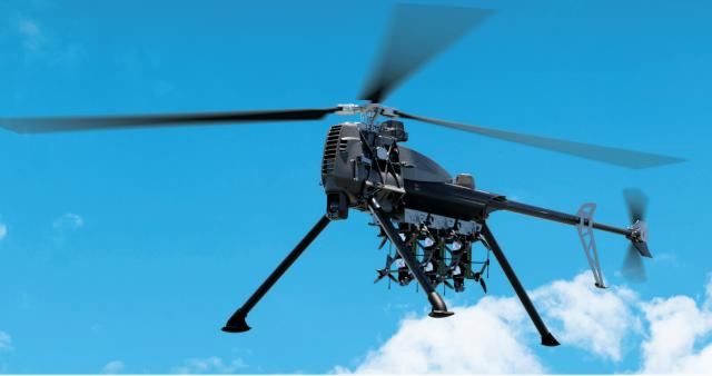
The TALON DT-150 is a very compact Group 2 unmanned aerial system (UAS) developed as a smaller counterpart to the TALON DT-300. Designed for versatility and portability, the DT-150 serves various applications, including reconnaissance, surveillance, and target acquisition as well as the ability to deliver useful logistics or three One Way Effect (OWE) explosive attack drones.
