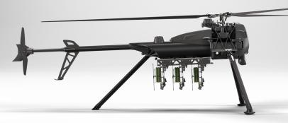
THE DT-150 CAN BE EQUIPPED WITH UP TO 3 DRONES OR ALTERNATIVELY CARRY UP TO 22.5KG / 50LBS OF CARGO BAGS
